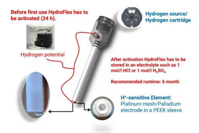
Before the first use the hydrogen electrode HydroFlex has to be activated thus the hydrogen production in the hydrogen generation cell is started. The arising hydrogen fills the PTFE-tube and leaks out of the platinum-palladium electrode where – according to the ions in the solution – a hydrogen potential sets. The hydrogen potential can be gripped on the gold-plated socket in the electrode's head. Once activated, the electrode works continuously for 6 months.
