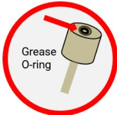
In the recess in the electrode head you see a small O-ring. Please grease this, e. g. with silicone grease.
