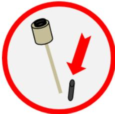
Remove the protective cap from the electrode carefully.
