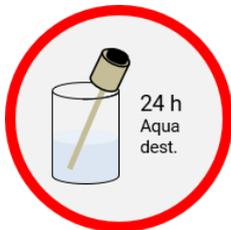
Place Mini-HydroFlex in water for 24 hours.
