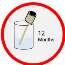
As soon as the running time of 12 months is reached, the hydrogen cell must be replaced immediately (see 4. Maintenance). Otherwise, a negative pressure will build up in the capillary so that liquid can get into the capillary.
