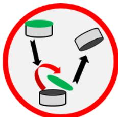
Take the replacement hydrogen cell and remove the protective foil. There are two openings visible. If any adhesive residue remains, remove it by rubbing with a cloth.
