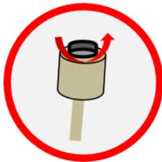
Unscrew the screw cap and remove the hydrogen cell.
