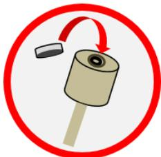
Insert the hydrogen cell with these two openings down into the recess.
