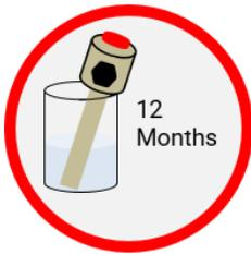
As soon as the running time of 12 months is reached, the hydrogen cells must be replaced immediately (see 5. Maintenance). Otherwise, a negative pressure will build up in the capillaries so that liquid can get into the capillaries.
