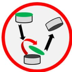
Take a new hydrogen cell and remove the protective foil. Two openings become visible. If any adhesive residue remains, remove it by rubbing with a cloth.
