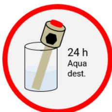
Place the hydrogen pH electrode in distilled water for 24 hours.
