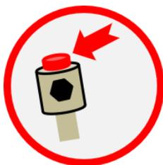
pHydrunio is already filled with internal electrolyte. Replace the red transport plug in the electrode head with the enclosed red pressure relief valve, which is also a screw cap.
