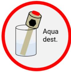
After the measurements, rinse the hydrogen pH electrode thoroughly with water. Please place the pH electrode in a vessel with distilled water. Under no circumstances it should be stored in the transport cap. The hydrogen would squeeze slowly the small volume of liquid out of the cap. The hydrogen pH electrode should not be stored dry in air as long as the hydrogen cells are generating hydrogen. A mixed potential forms which can lead to incorrect results.
