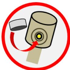
Place one hydrogen cell in the recess with these openings facing down.
