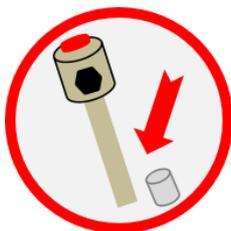
Carefully remove the transport cap from the bottom of the electrode shaft.
