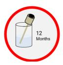
As soon as the runtime of 12 months is reached, the hydrogen cell must be replaced immediately (see 4. Maintenance). Otherwise, a negative pressure will build up in the capillary so that liquid can get into the capillary.
