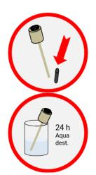
Remove the protective cap from the electrode carefully.
