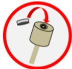
Insert the hydrogen cell with these two openings down into the recess.
