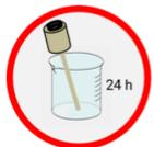
Place Mini-HydroFlex in water for 24 hours.
