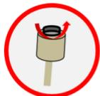
Unscrew the black cap and remove the hydrogen cell.
