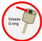
In the recess in the electrode head you see a small o-ring. Please grease this, e.g. with silicone grease.
