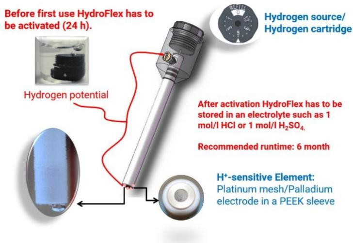
Before the first use the hydrogen electrode HydroFlex has to be activated thus the hydrogen production in the hydrogen generation cell is started. The arising hydrogen fills the PTFE-tube and leaks out of the platinum-palladium electrode where – according to the ions in the solution – a hydrogen potential sets. The hydrogen potential can be gripped on the gold-plated socket in the electrode's head. Once activated, the electrode works continuously for 6 months.
