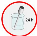
Place Hydroflex for 24 hours in the water. At least half of the shaft should be surrounded by water.
