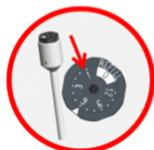
On top of the electrode head turn the runtime clockwise to position 1 with a 3 mm hex screw driver. That is corresponding to one month.
