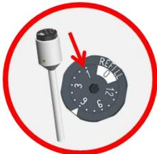
On top of the electrode head turn the runtime clockwise to position 1 with a 3 mm hex screw driver. That is corresponding to one month.
